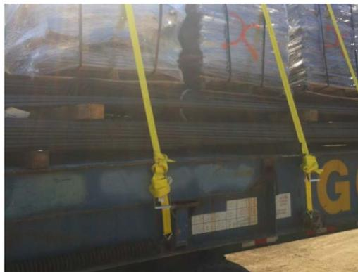
**Improperly secured load: should have had multi-level strap lashings, bottom with chain binders and top with straps. Please note the cargo on each pallet is also lashed through the pallet.**
