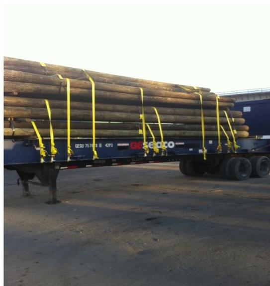
**Properly strapped multilevel load**
